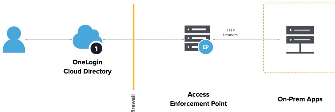
High-level architecture of OneLogin Access, which provides user session information and access control services to applications hosted on premises, at data centers, and in private clouds.
